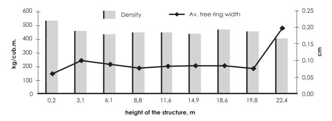
Figure 3. Properties of timber used for the building of the Church of the Transfiguration
